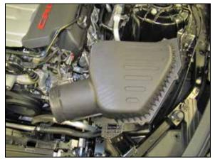
12. Remove the factory air filter housing from the vehicle.
