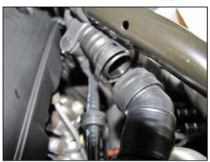
9. Disconnect the sound tube quick disconnect and then remove the complete sound tube assembly.
