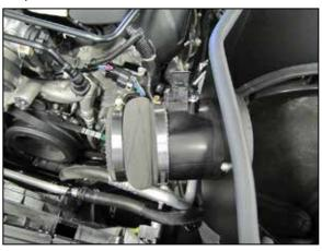
19. Install the provided hump coupler (08633) onto the mass air sensor housing and secure with the provided hose clamps.
