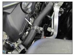
7. Open the clamp that secures the sound tube to the factory air filter housing.
