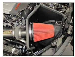
24. Install the AEM® air filter and secure with the provided hose clamp.
