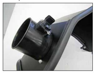
16. Remove the mass air sensor from the factory air filter housing and install it into the AEM® air filter housing using the provided hardware.
