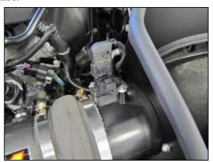
23. Reconnect the mass air sensor electrical connection.
