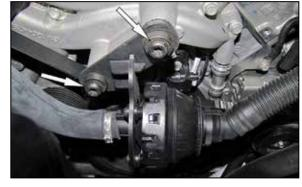
6. Remove the two bolts that secure the sound drum to the engine.
