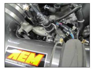
22. Connect the factory crank case vent line to the quick connect fitting installed into the AEM® intake tube.
