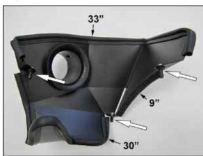
15. Install the edge trim onto the heat shield. Install the three provided mounting studs using the hardware provided.
