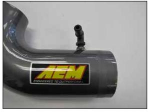
20. Install the  $90^{\text{o}}$  vent fitting into the AEM  $^{\!\! 8}$  intake tube as shown.
