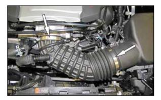
5. Loosen the hose clamps that secure the factory intake tube and then remove the intake tube from the vehicle.
