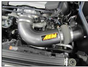
21. Install the AEM® intake tube into the hump coupler and then into the coupler at the throttle body, adjust the tube for best fit and then secure with the provided hose clamps.
