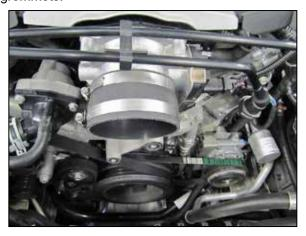
18. Install the provided coupler (08761) onto the throttle body and secure with the provided hose clamps.
